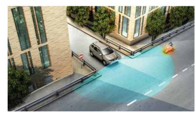
**MultiView Camera.\*** Connected to the MediaNav system, the MultiView Camera shows the images from Duster's four on-board cameras. It is triggered by reverse gear or by a simple touch of the dedicated button. \*Standard on 4x4 and Intens model
