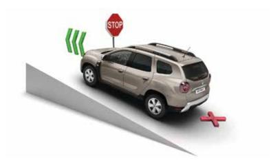
**(HSA) Hill Start Assist.** Starting the car on steep slopes is no longer a worry. When you take your foot off the brake, hill-starting assist takes over and holds the vehicle steady for two seconds. This gives you time to accelerate normally without stalling or rolling back.
